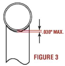
Filling or bridging gaps will result in weak joints as high stresses are generated when the weld pulls the joint together. The smaller the gap, the lower the stress, the stronger the joints. Again, use holding blocks mentioned in handling section. (Figure 1)
